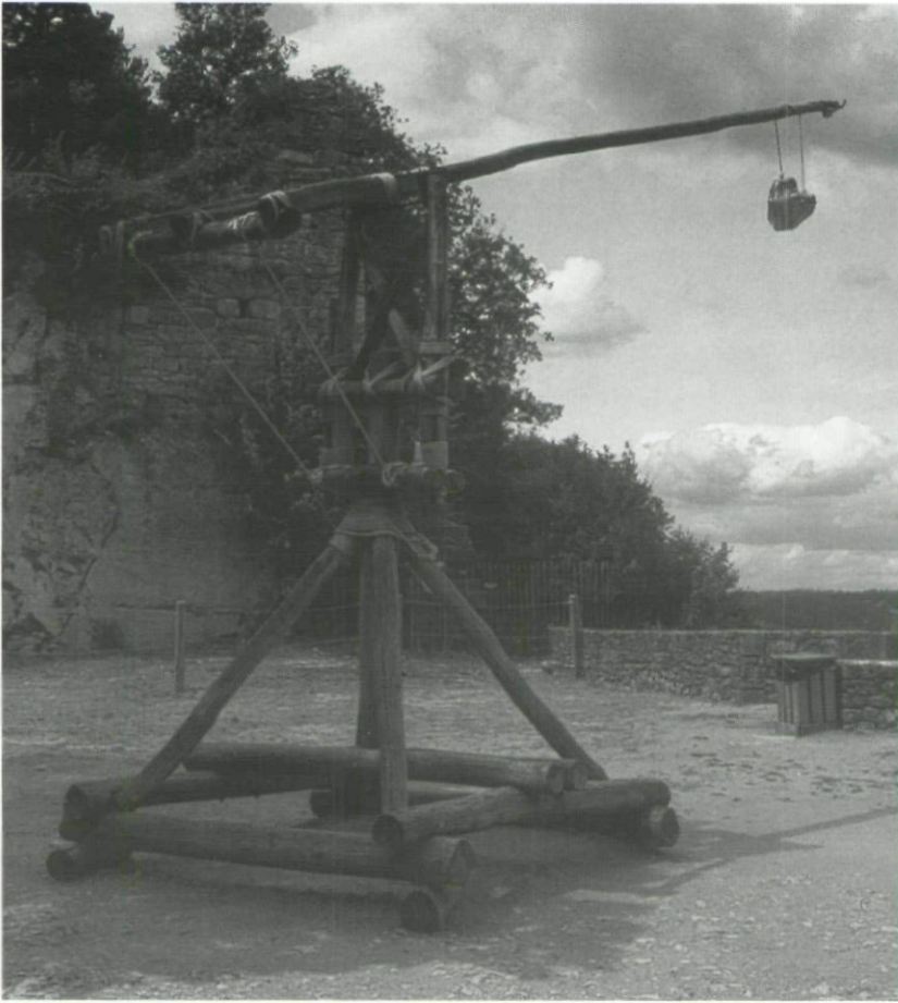
Figure 1 Reconstruction of a medieval mangonel at Castelnaud (Dordogne) that is representative of the manually propelled stone thrower (perrier) in common use throughout the medieval period. Author's photograph.
