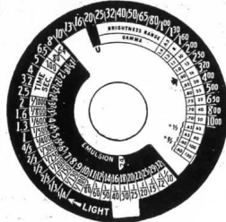
Fig. 3. Proper dial setting for the scene of average brightness range above.
