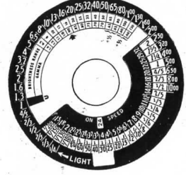
Fig. 2. Exposure meter dial with supplementary dial.
